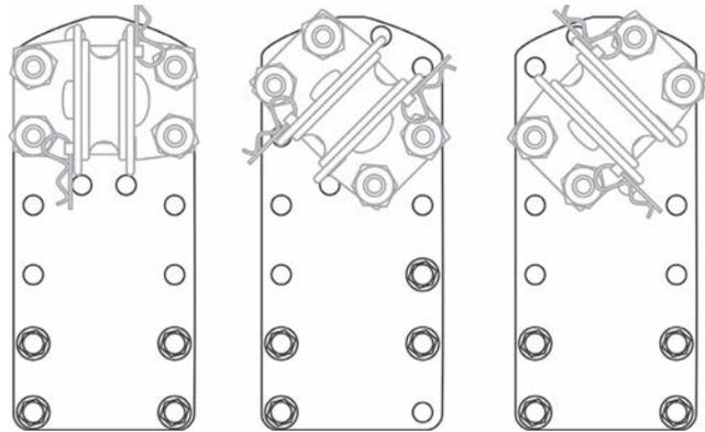
The pulley (not included) can be rotated in three different ways, as shown above. Use any of the eight mounting holes, based on the application.
